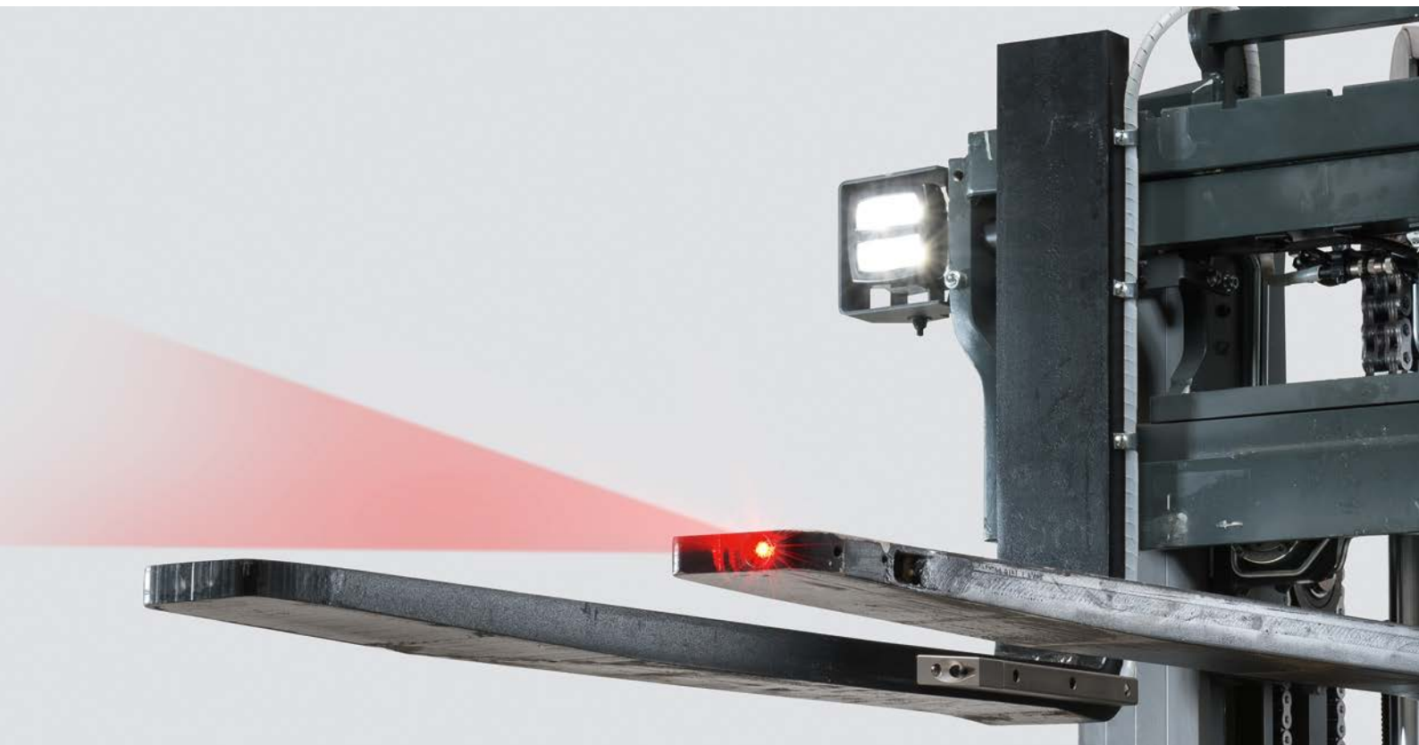
LED spotlights on fork carriages and positioning laser
