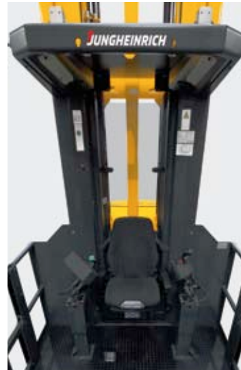
EKX 515, split operator consoles and conversion to a picking truck
