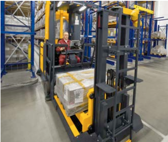
EKX 513, telescopic fork with auxiliary lift in front of the fork and emergency escape ladder
