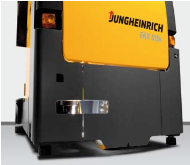
Protected laser scanner in an EKX 515k
