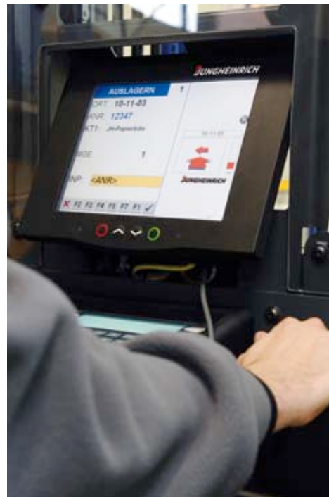
The "Route guide" shows the driver the direction and route
