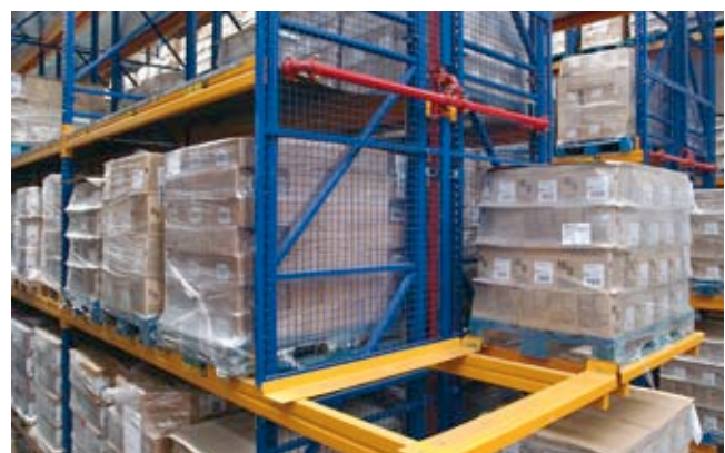
P&D location with projecting bearing surfaces
