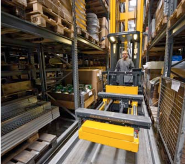
EKX 515, hydraulically adjustable telescopic fork
