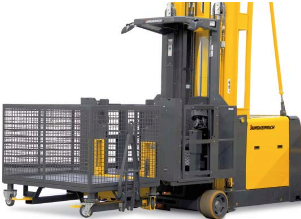
Lower cut out for a picking cage
