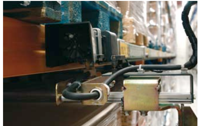
Enclosed conductor rail with current collector
