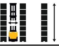
1.8 m Aisle width 17.5 m Lift height
