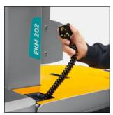
On-board charger with integrated spiral cable
