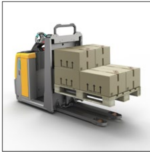
Easily lifting load section for order picking at an ergonomic height
