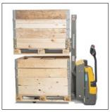
Double-deck operation: Loading of two pallets one above the other
