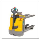
Short mast of the EMD 115i for ergonomic order picking up to a height of 690 mm
